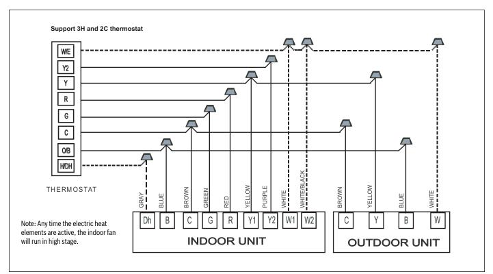
Figure 25 Thermostat Wiring Diagram for BOVA2.0/BVA2.0 Matched System
