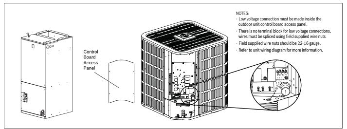
Figure 24 Low Voltage Unit Connections
