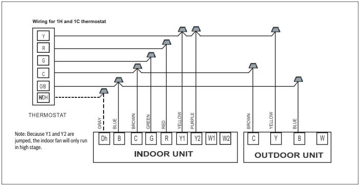
Figure 29 Thermostat Wiring Diagram for BOVA2.0/BVA2.0 Matched System
