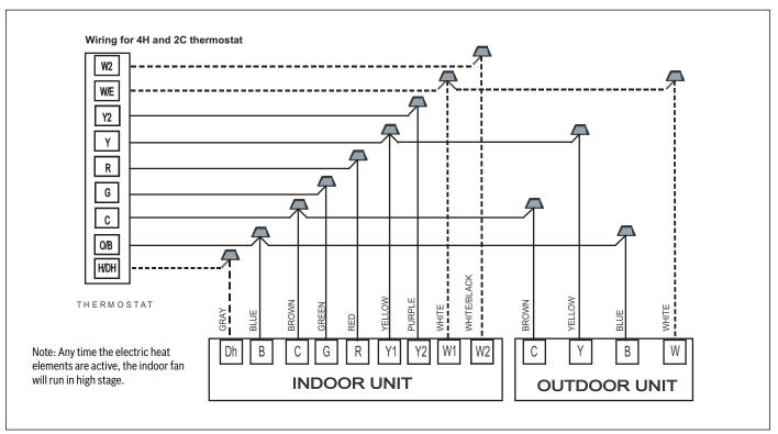
Figure 26 Thermostat Wiring Diagram for BOVA2.0/BVA2.0 Matched System
