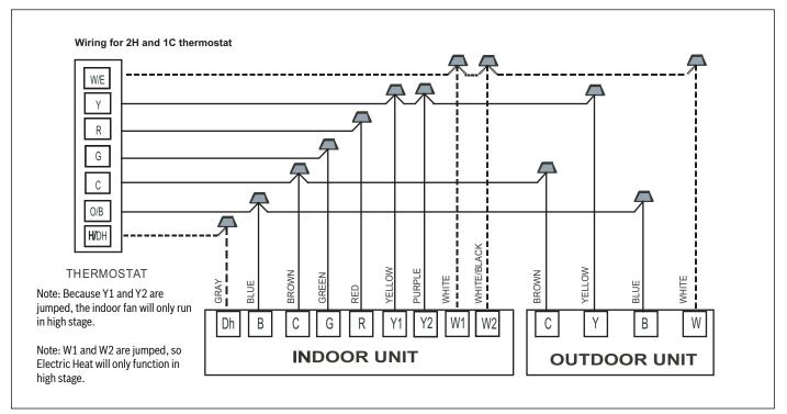
Figure 30 Thermostat Wiring Diagram for BOVA2.0/BVA2.0 Matched System
